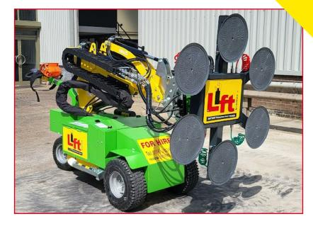
The new GW625-2 is perfect for building projects with large window sections which require a large load bearing capacity of up to 625kg.
